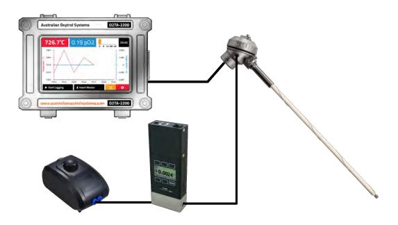
Ideal electrical interface to the probe will have the following characteristics, and include a diaphragm air pump to supply the clean reference air.
