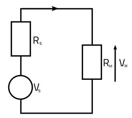
Calculating the system current to be defined as  $i=\frac{V_s}{(R_s+R_M)}$ , the voltage seen by the measurement equipment will then be  $V_M=i\cdot R_M$ . In this instance the measurement voltage will be –19.3 mV, approximately half the sensor unloaded voltage.
