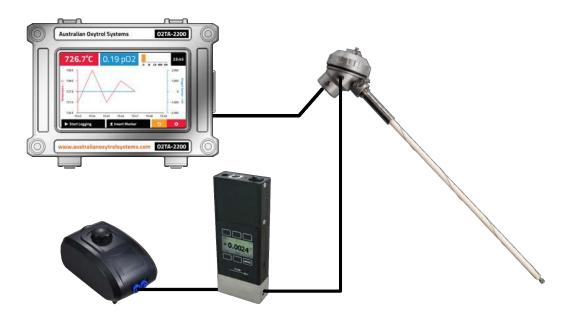
Ideal electrical interface to the probe will have the following characteristics, and include a diaphragm air pump to supply the clean reference air.
