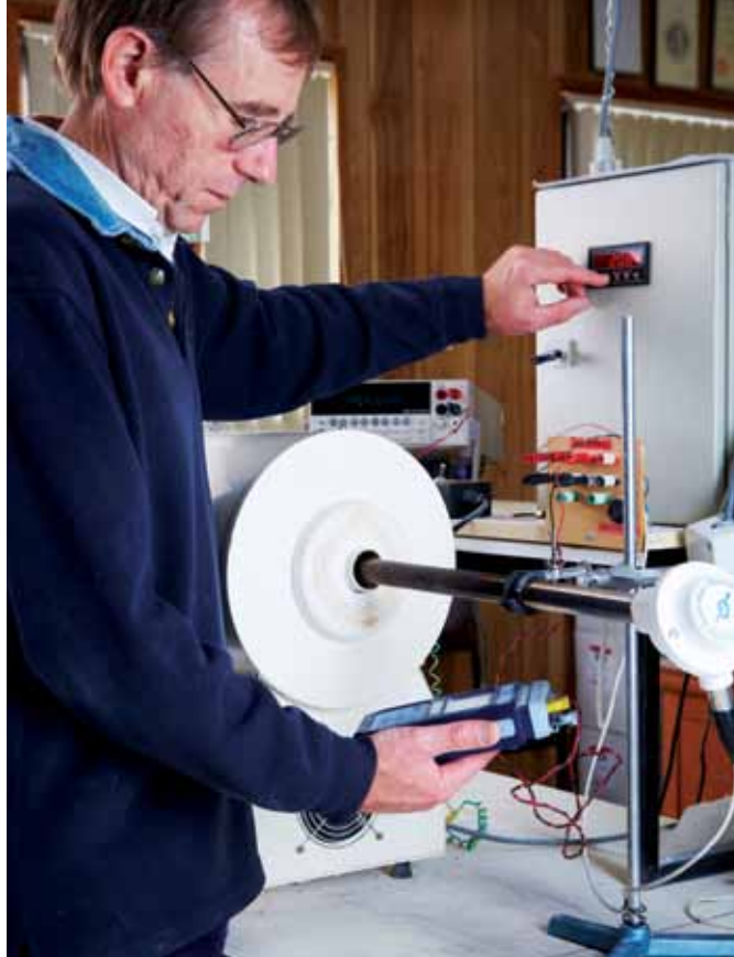
Above Middle: Checking an oxygen probe in our test and calibration facility.
