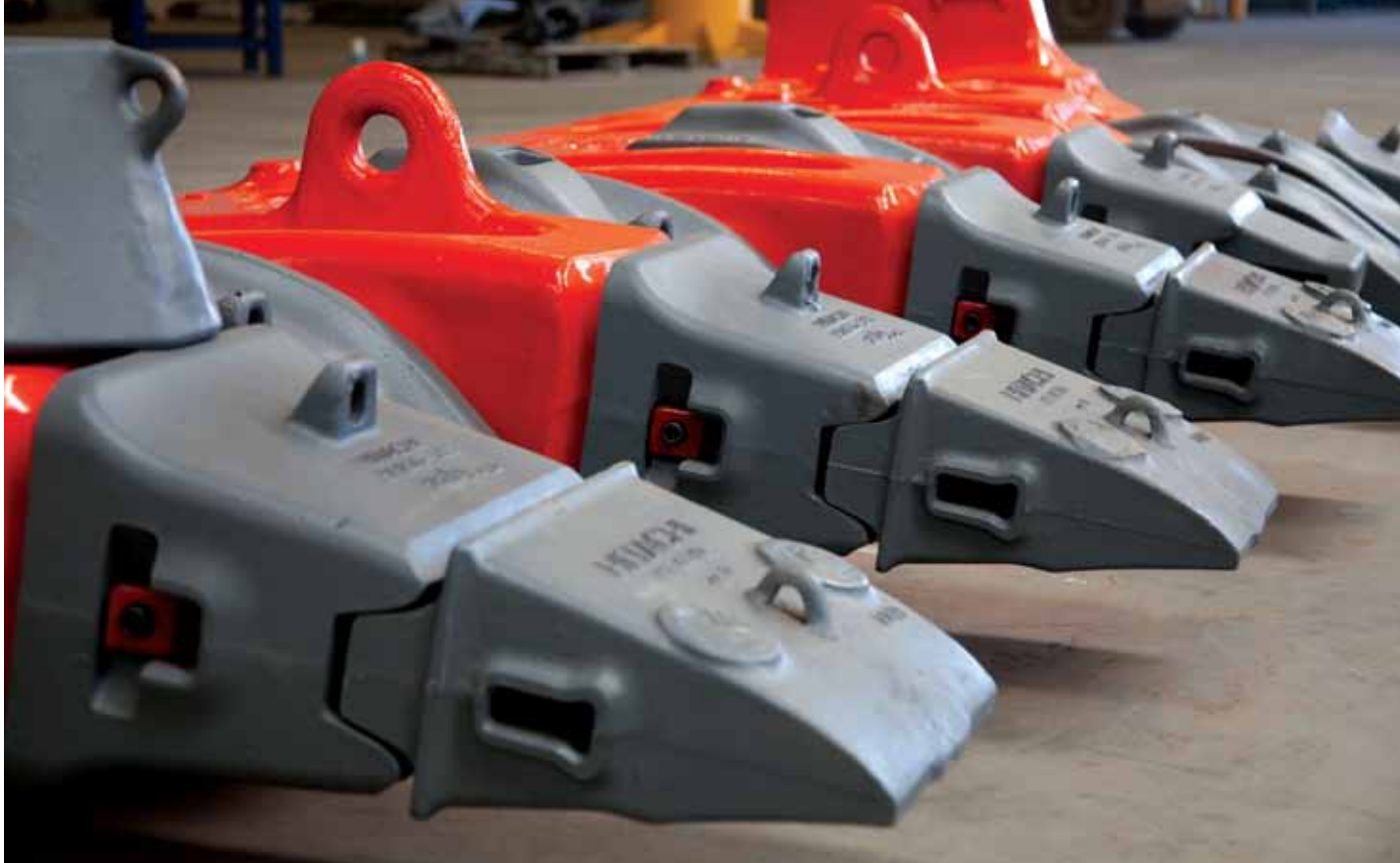
Left: The Keech Moonlock™ crusher and ore bin quick changeover wear protection system is extremely flexible.
